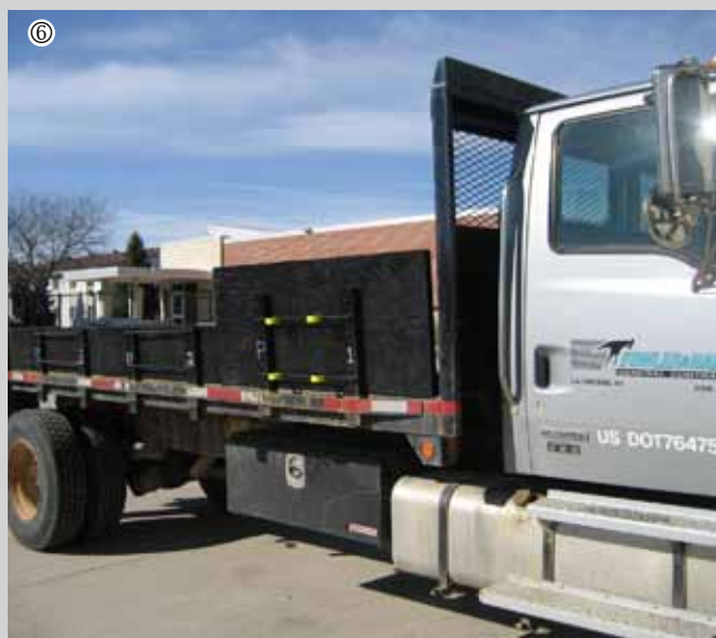
4. Pete Harris grinding floors at the Kumm Center. 5. Ike and Sue working at the office. 6. New sides installed on the truck, making it less likely to be overloaded in the future.
